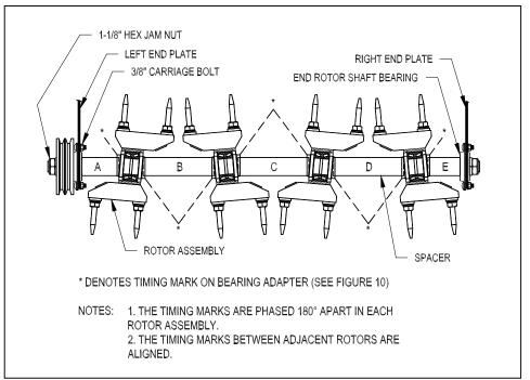
Figure 6. Rotor Shaft Assembly
